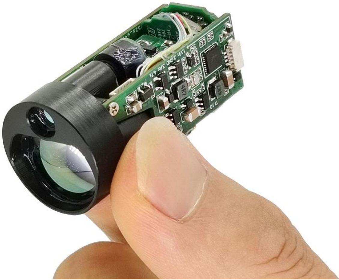
JIO-M010X miniature laser rangefinder module adopts 905nm semiconductor laser components, with low power consumption, small size, stable performance and other characteristics, suitable for thermal imaging, night vision and other handheld mobile devices and miniaturized UAV pod equipment integration.
