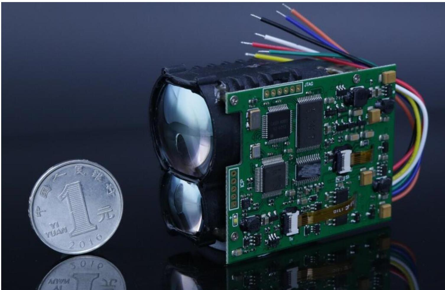
JIO-M40X miniature laser rangefinder module adopts 905nm semiconductor laser components, with low power consumption, small size, stable performance and other characteristics, suitable for thermal imaging, night vision and other handheld mobile devices and miniaturized UAV pod equipment integration.
